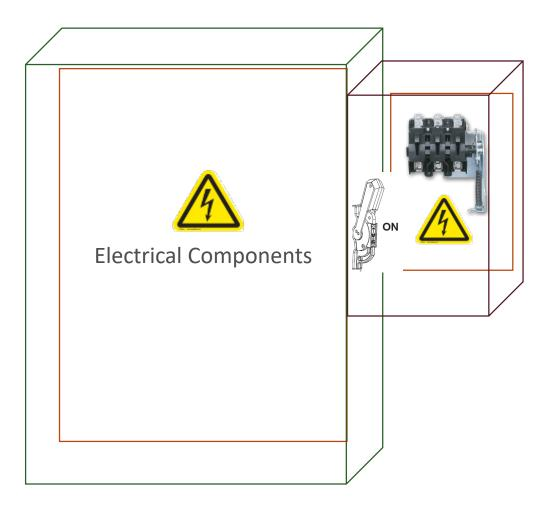
When the disconnect handle is in the OFF position, the hazard is removed downstream of disconnect (Load Side). This eliminates the hazard and risk of electrical shock or arc flash by accidental contact in the main enclosures. Line side voltage hazard is still present inside Sequestr
